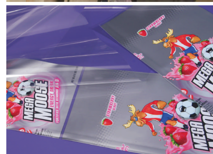
A quality check, above, assures the film's printing registration and integrity.
