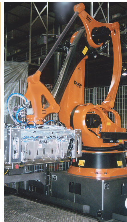
The carbon-fiber-composite robotic arm demonstrates extremely high stiffness characteristics that enable it to stack loads weighing up to 180 kg to heights up to 3 m.
